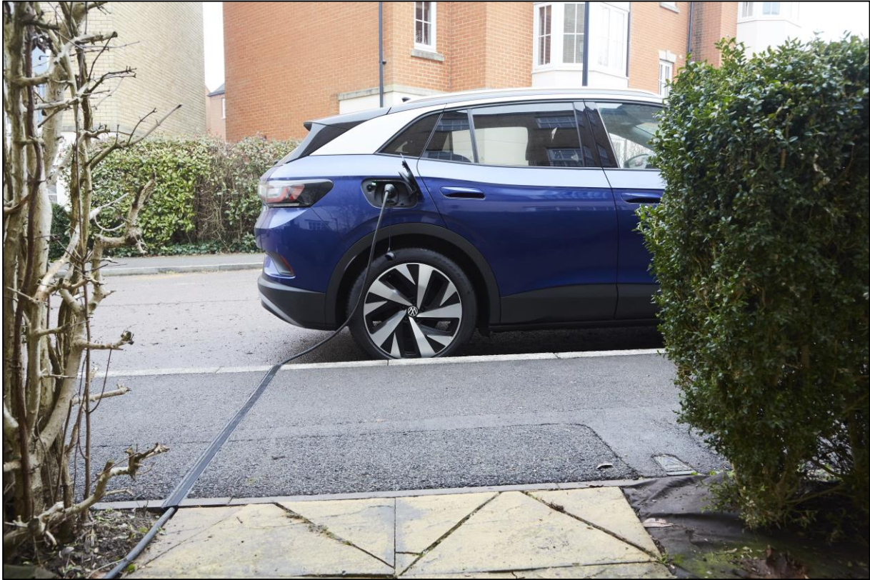
Figure 17: A vehicle charging using the pavement cable channel offered by Kerbo Charge
