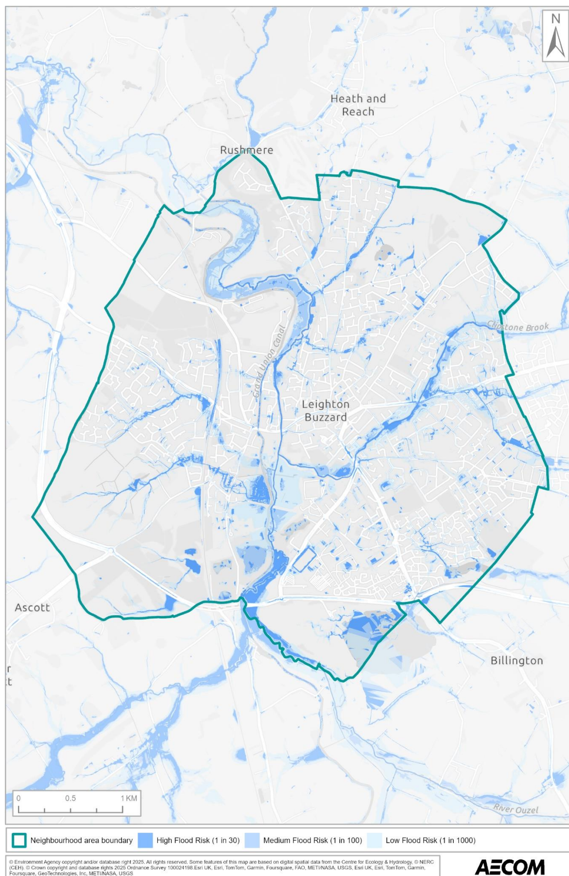
Figure 4-4: Surface water flood risk in Leighton-Linslade
